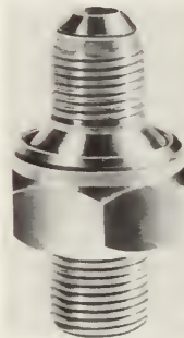
20-7. A safety head (ruptured disc type) for Freon-12. The disc is made of silver. The safety head is obtainable having various rupture pressures from 175 psig to 1000 psig. The safety head is usually designed to rupture at 50 per cent above the usual operating pressure.
